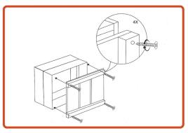
Place the bottom piece in (it should fit snug inside!) and screw the four larger screws into the wood slats.
