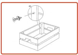
With the enthusiasm of an Easter egg hunt, use a manual screwdriver to screw the 4 shorter screws into the sides to connect.
