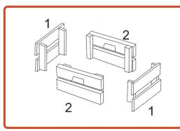
Start by placing the four sides together, ensuring the handles are on the top panel.
